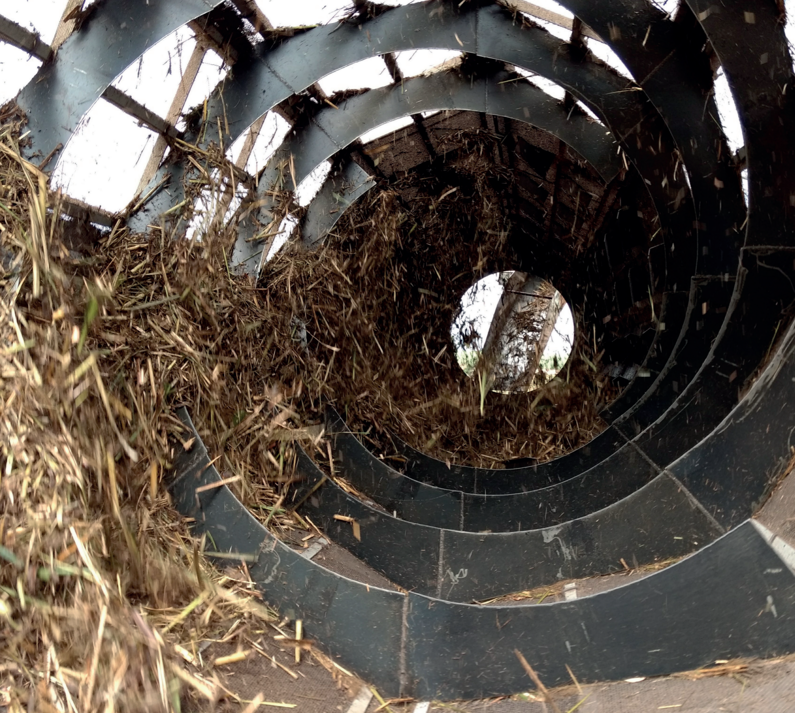
Rotary sieve straw screening
