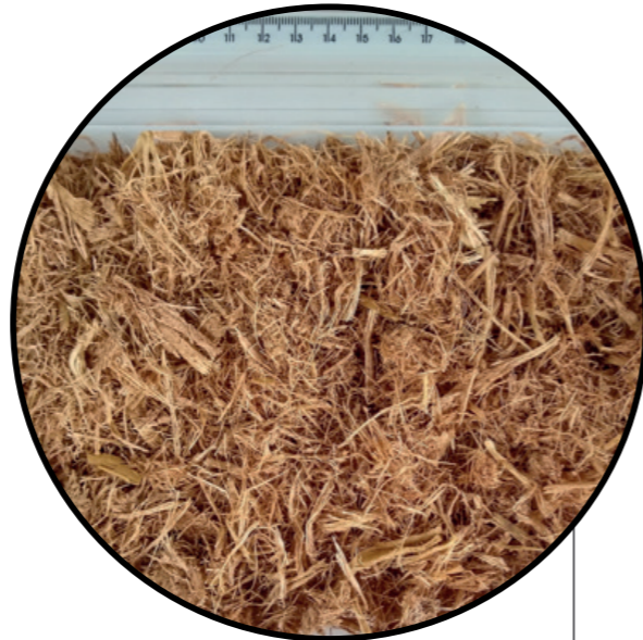
Crushed straw and bagasse mixture aspect from the last mill in the tandem
