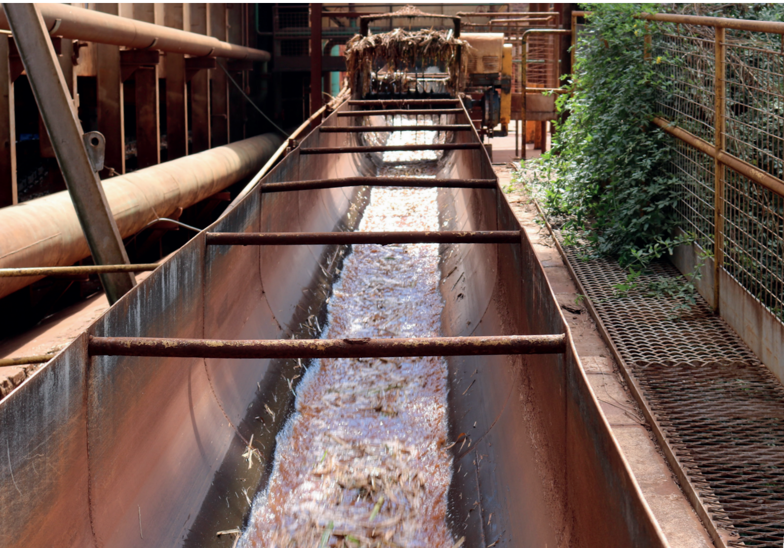
Straw washing into the channel
