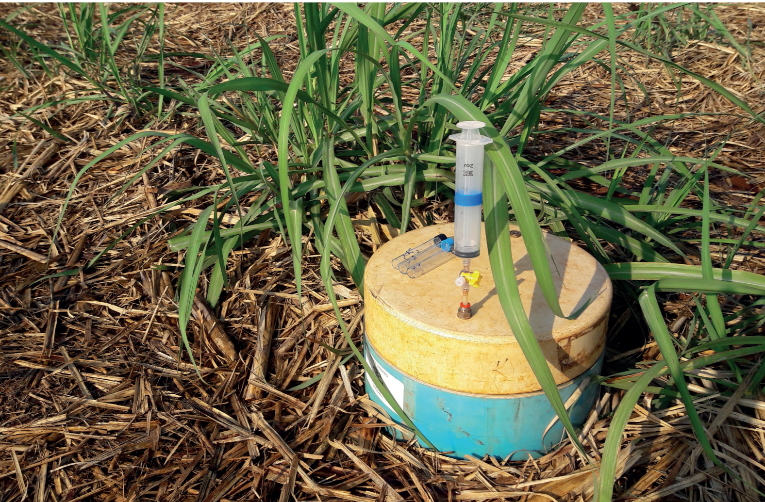
Experiment for collecting greenhouse gas emissions
