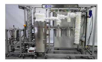
The equipment is designed for analyzing the main parameters of gasification and pyrolysis processes of solid and liquid fuels and residues. The reactor is of the bubbling fluidized bed type with continuous feed flow in the order of 1 - 2 kg / h and it has a temperature control system, where the set points are keeped by the action of electrical resistances that heat the gasification agents, reactor, cyclone and hot metallic gas filter
