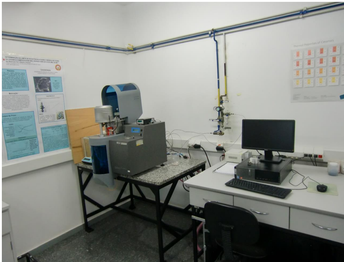
Calorimeter (DSC) with thermogravimetric analysis (TG) - (LC3).
